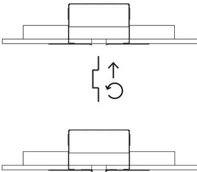
Position Alignment Gauge (provided with all Straight and End Modules) between perforated screens to ensure even spacing before fastening the Maggy module into the drywall using self-tapping screws.
