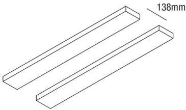
Frame desired location of Maggy module with 2x4 blocking to ensure proper fastening through drywall.
