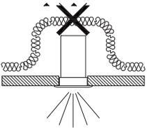
Fixtures not suitable to be covered in thermally-insulating material.
