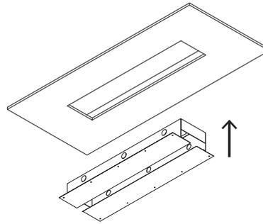
Install drywall and make a hole between blocking for placement of Maggy module.
