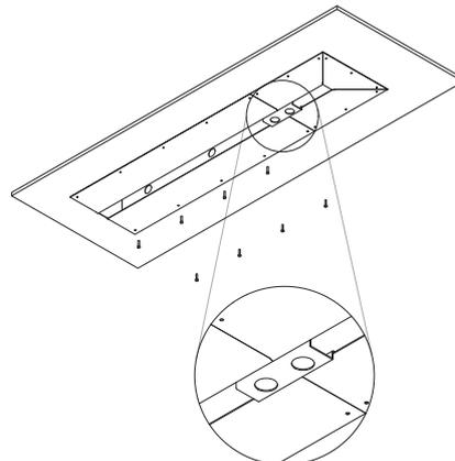
Use Alignment Gauge when joining two sections of Maggy module end to end to make clean, straight lines between two sections before plastering.
