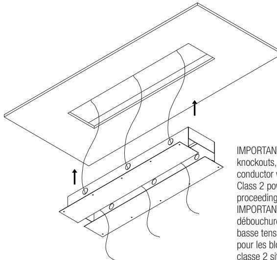
IMPORTANT: Using the 7/8" knockouts, pull 16/2 low-voltage 2 conductor wire for remote located Class 2 power supplies before proceeding.
